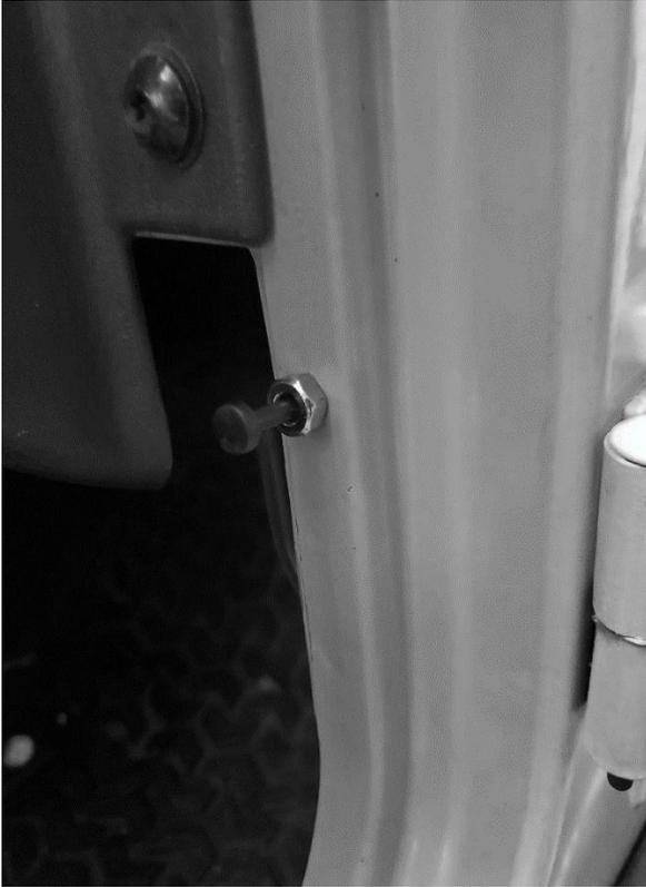
Route the wires from the control module to each switch and secure. The Brown wire connects to Drivers-side Door jamb switch and the Orange wire connects to the Passenger side door jamb switch.
