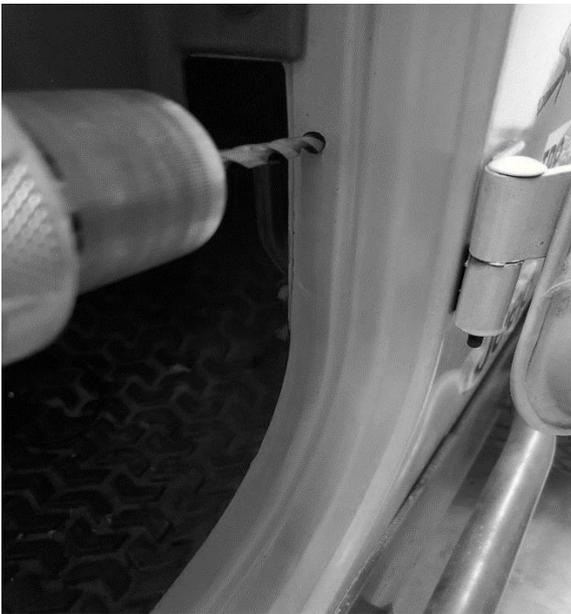
Locate a flat surface with no obstruction behind for the door jamb switches. Drill a pilot hole and then a 5/16" hole to mount each switch. Install using the washer and nut on the backside and tighten.
