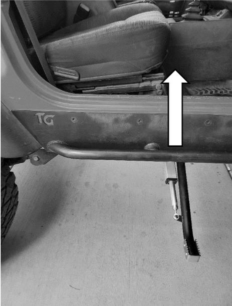
*Install the Zstep below the front edge of seat.*
